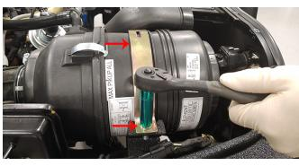
Remove breather hose, loosen clamp and remove air filter housing.
