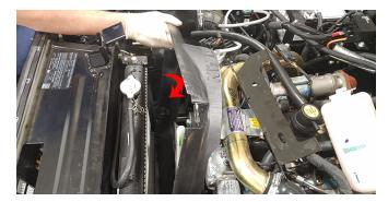
6. Remove M8 lower radiator core support fasteners. Retain fasteners for reuse.
