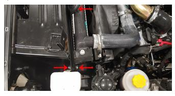
On opposite side, remove cable tie mount from bolt and set differential breather hose aside.
