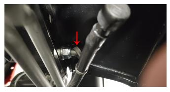
10. Remove M8 radiator core support fasteners. Retain fasteners for reuse.
