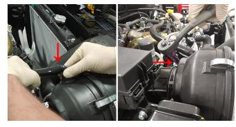
3. Remove (4) M8 nuts with washers and remove (2) upper radiator core support bars.
