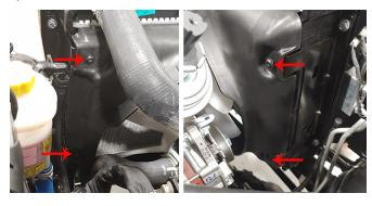
14. Re-install (2) radiator core support bars with (4) M8 nuts and torque to specification.
