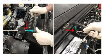
Counter-holding, remove M8 radiator core fasteners and remove coolant overflow bottle. Retain fasteners for reuse.
