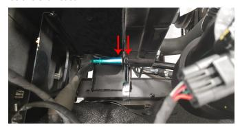
7. Install (2) U-nuts onto left fan shroud bracket. Re-using lower radiator core support fasteners, install fan shroud bracket.
