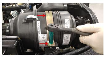
Re-install breather hose and tighten clamp for air filter housing.
