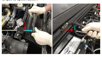
15. Re-using (1) M8 hex bolt, re-install air filter housing with bracket and torque to specification.
